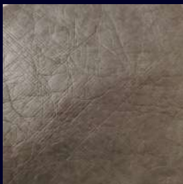
Material: Tyvek with PU coating
